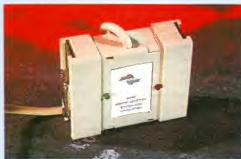
The Autoswitch from Alfa Data swaps between mouse and joystick as soon as you press a button on either.
